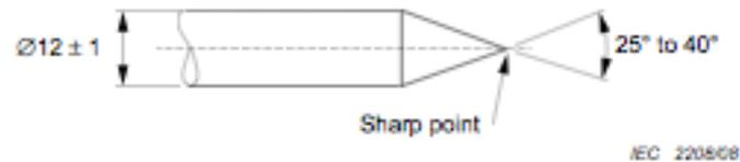
3b) – Discharge electrode for contact discharges
