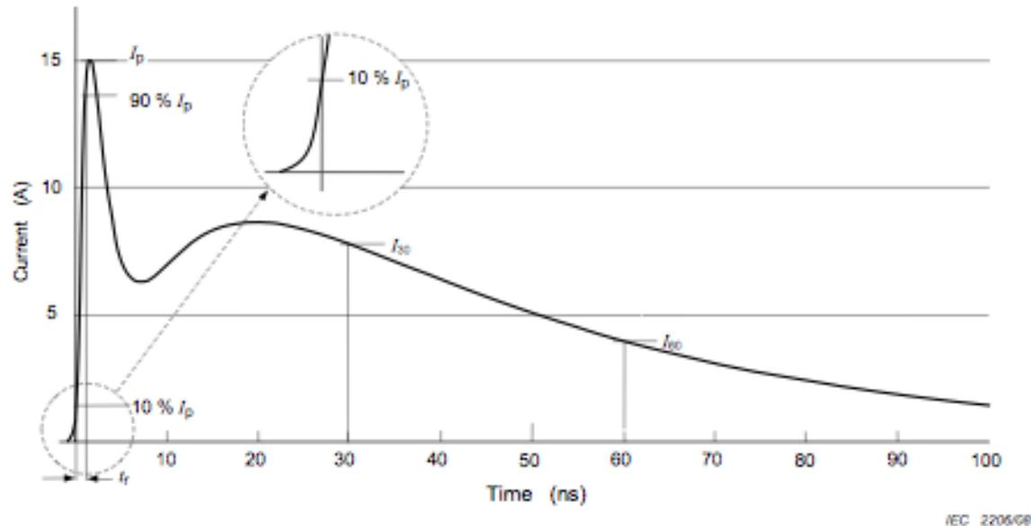
Figure 2 – Ideal contact discharge current waveform at 4 kV
