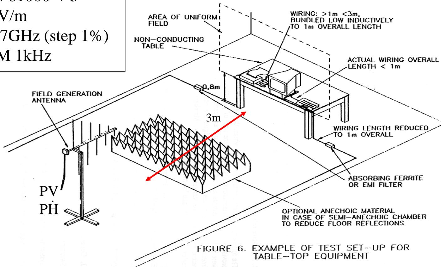
FIGURE 6. EXAMPLE OF TEST SET-UP FOR TABLE-TOP EQUIPMENT
