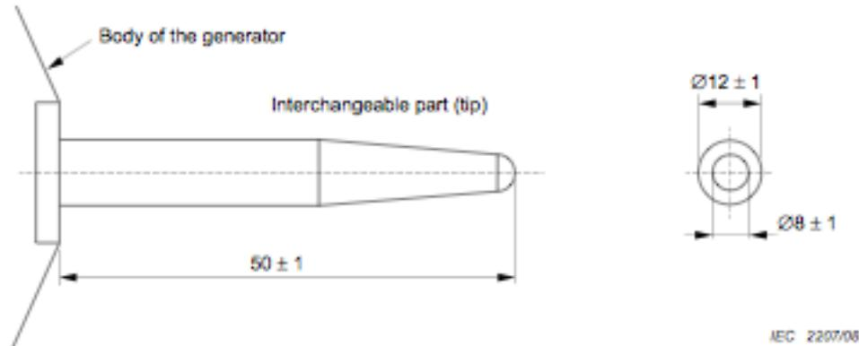
3a) – Discharge electrode for air discharges
