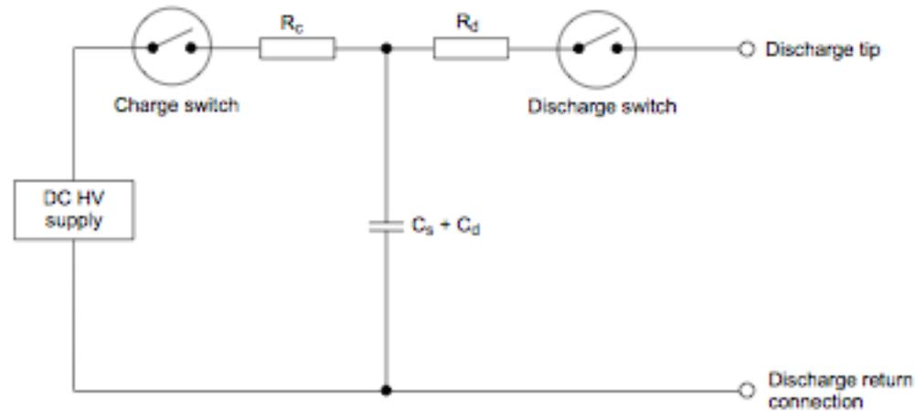
NOTE 1  $C_d$  is a distributed capacitance which exists between the generator and its surroundings.
