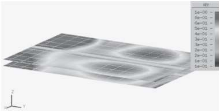
Figure 9.247. With only one stitching post at the left-hand I/O area, high levels of ESD pulse reflections are observed. (Courtesy of Dr. Bruce Archambeault.)
