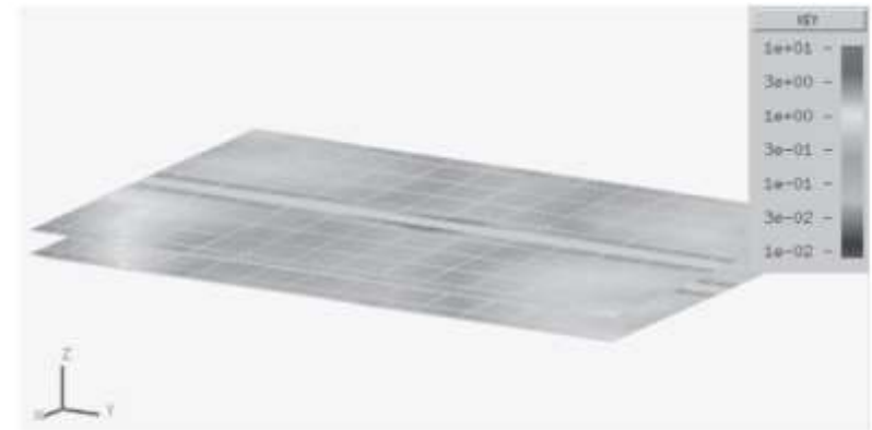
Figure 9.249. With four stitching posts placed at both ends of the PCB, lower levels of ESD pulse reflections are observed but propagation across the PCB still occurs. (Courtesy of Dr. Bruce Archambeault.)
