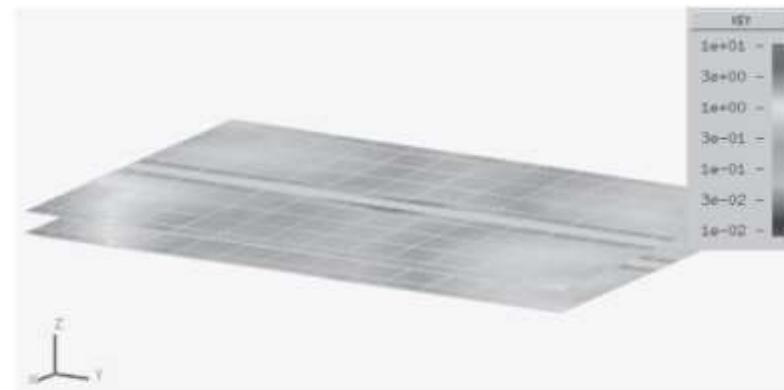
Figure 9.247. With only one stitching post at the left-hand I/O area, high levels of ESD pulse reflections are observed. (Courtesy of Dr. Bruce Archambeault.)
