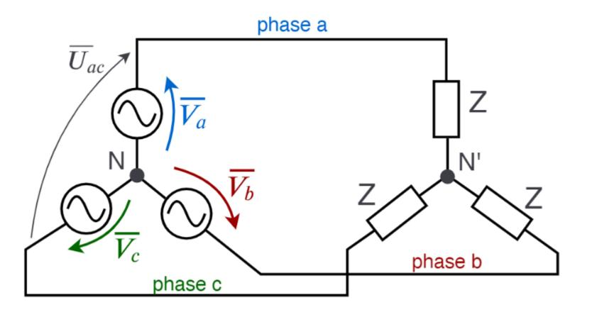
The balanced three-phase circuit is the assembly of three identical circuits called phases. The 3 signals are dephased by 120°.
