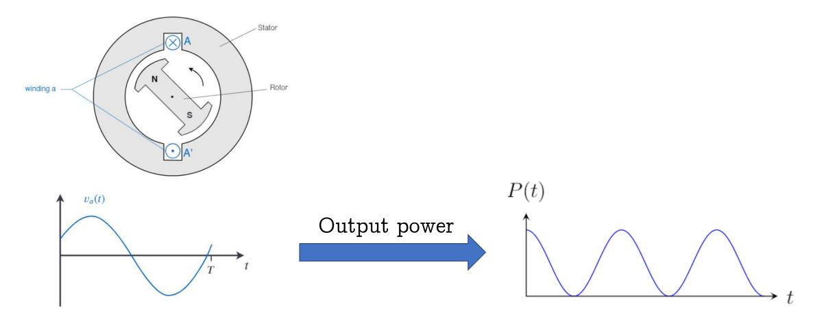
The total output power fluctuates  $\rightarrow$  the input torque fluctuates  $\otimes$
