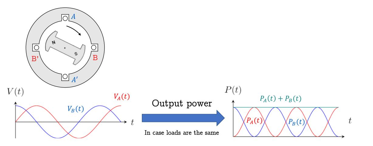
• The total output power is constant  $\rightarrow$  the input torque is constant  $\odot$
