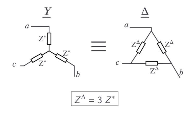
From the network perspective, the Y and  $\Delta$ arrangements ae equivalent as long as they provide the same line voltages and current. This is achieved in case  $Z^{\Delta} = 3 Z^*$ .
