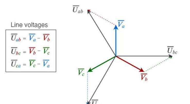
$\overline{V}_a$ ,  $\overline{V}_b$  and  $\overline{V}_c$  are the phase voltages, measured between a phase and the neutral N.
