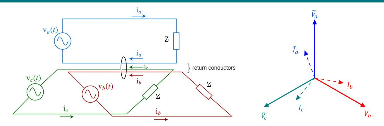
$\bar{I}_a + \bar{I}_c + \bar{I}_c = 0$  (for identical load Z) The 3 return conductors can be removed  $\odot \odot \odot$
