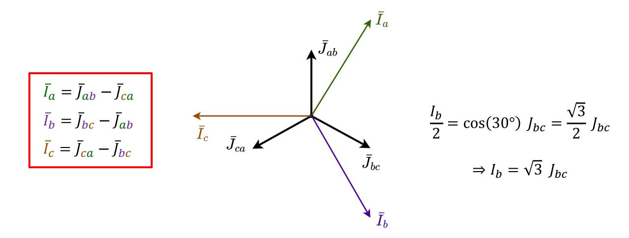
In a delta configuration, the line current is  $\sqrt{3}$  the phase current.
