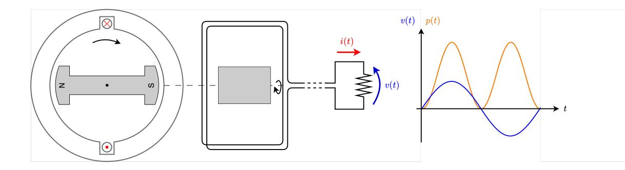
The output power p(t) fluctuates so that the input torque fluctuates as well. However, we would like to have a constant input torque.
