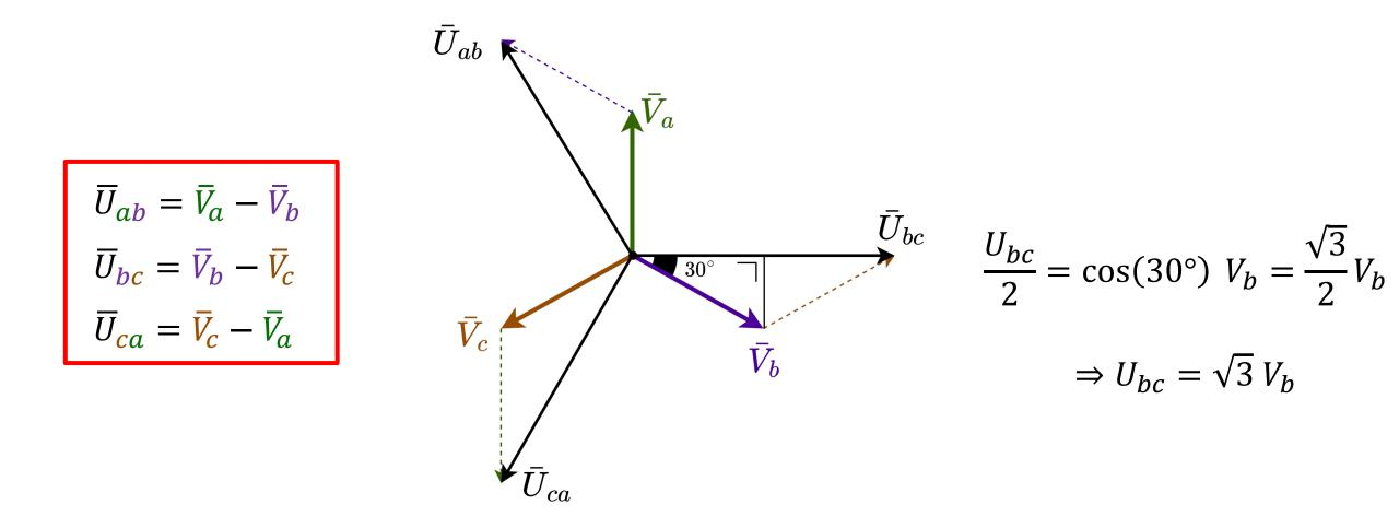
In a star configuration, the line voltage is  $\sqrt{3}$  the phase voltage.
