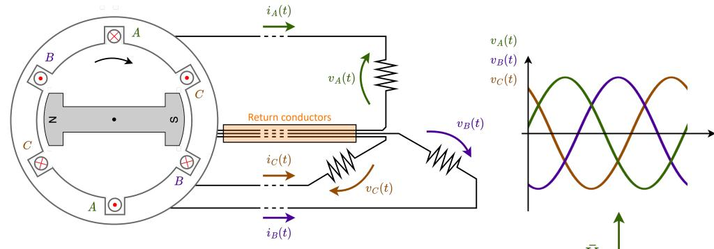
Using identical loads, the input torque also remains constant when using three phases. Moreover, plotting the current phase diagram, it appears that the sum of the currents is zero. The return wires can thus be removed.
