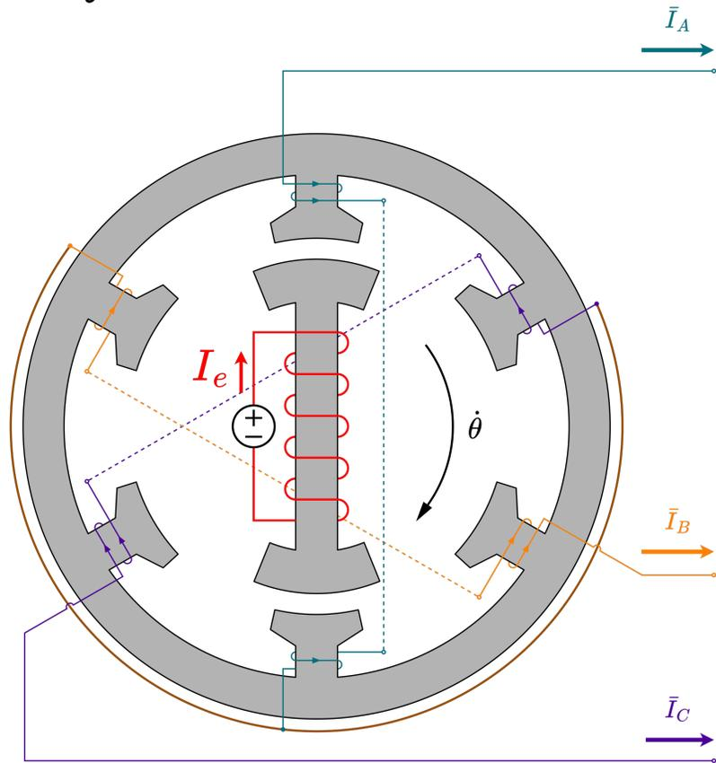
An electromagnet generates a flux  $\phi(I_e)$ , rotating with the shaft of the machine.
