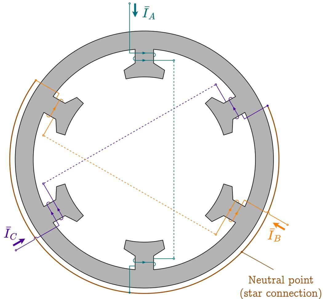
It is powered by a balanced three-phase electrical grid so that the currents  $\bar{I}_A$ ,  $\bar{I}_B$  and  $\bar{I}_C$  are out of phase by  $120^\circ$  and have equal peak amplitude  $I_p$ .
