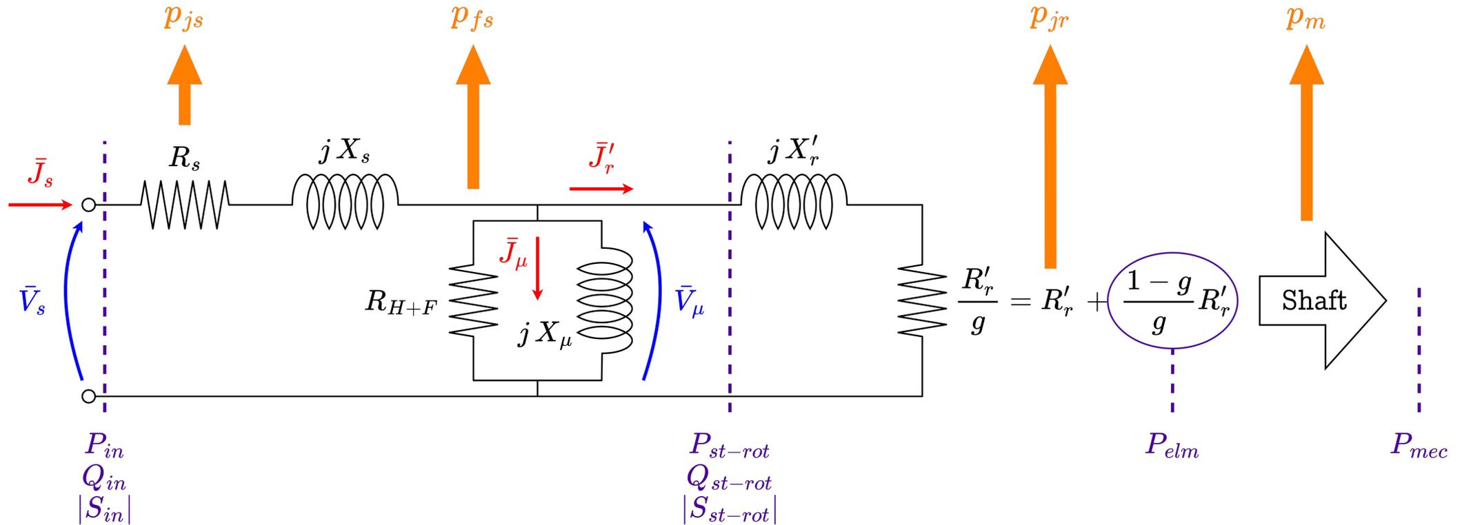
Power transmitted from the stator to the rotor:  $P_{st-rot} = P_{in} - p_{js} - p_{fs} = P_{in} - R_s J_s^2 - \frac{V_\mu^2}{R_{H+F}}$
