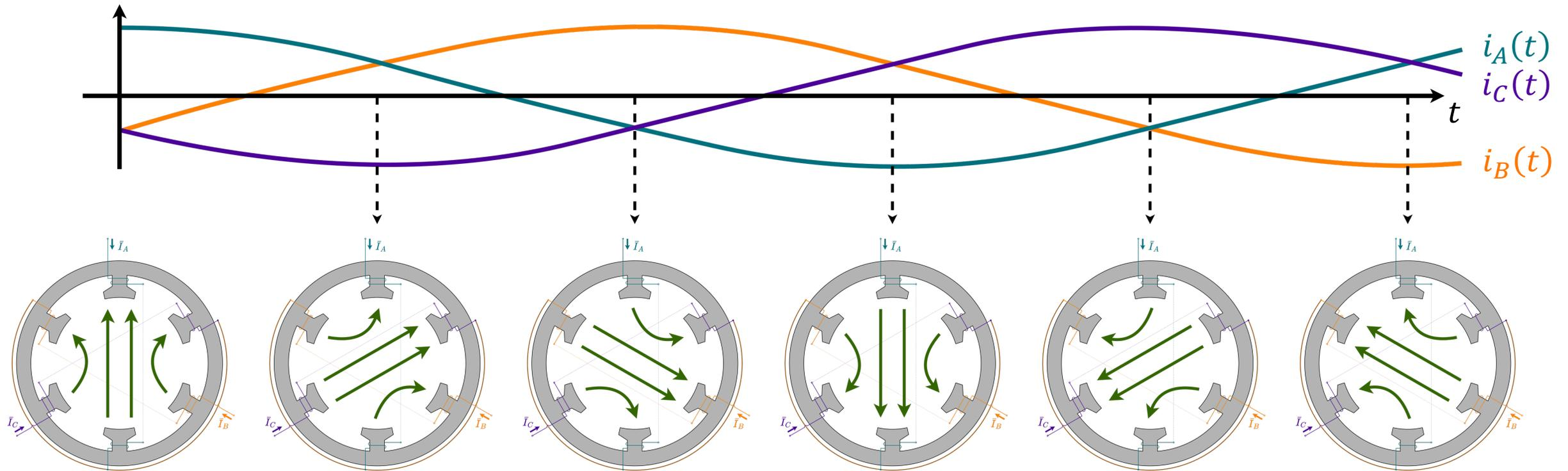
The magnetic field generated in the stator is constant in amplitude and rotates at the frequency of the three-phase power source.
