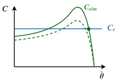
→ Modifying the voltage has a very small impact on the rotation speed.
