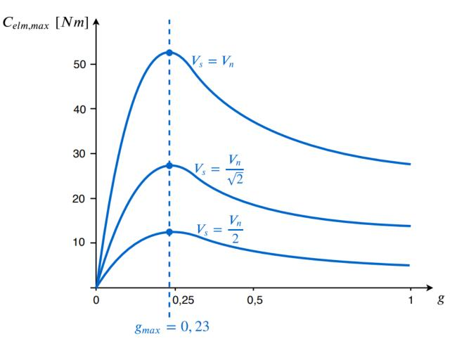
12. Explain why a control on the rotor voltages is not suitable for speed variation for load having constant resistive torque.
