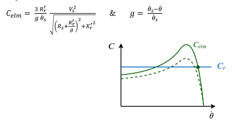
→ Modifying the voltage has a very small impact on the rotation speed.
