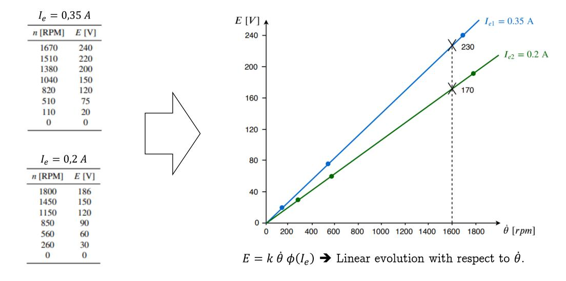
2. Show that the flux  $\Phi$  is not proportional to the excitation current intensity  $I_e$ .
