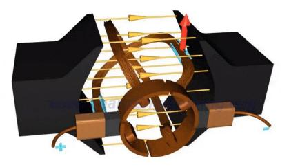
The stator generates a constant magnetic field.
