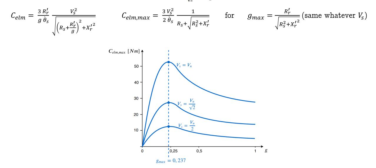
Explain why a control on the rotor voltages is not suitable for speed variation for load having constant resistive torque;
