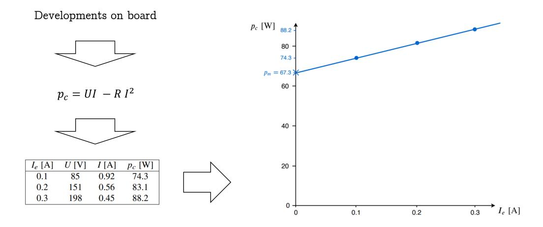
6. For the linear part of the curve, determine the mechanical losses  $p_m$  at the nominal speed of rotation.
