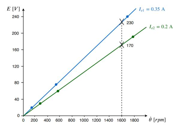
The excitation current  $I_{e1}$  is  $\frac{I_{e1}}{I_{e2}} = \frac{0.35}{0.2} = 1,75$  times the excitation current  $I_{e2}$ .
