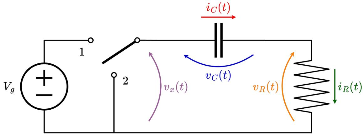
$$\left. \begin{aligned} v_x(t) &= v_C(t) + v_R(t) \\ i_C(t) &= i(t) = C \frac{dv_C(t)}{dt} \\ i_R(t) &= i(t) = \frac{v_R(t)}{R} \end{aligned} \right\} C \frac{dv_C(t)}{dt} = \frac{v_x(t) - v_C(t)}{R}$$
