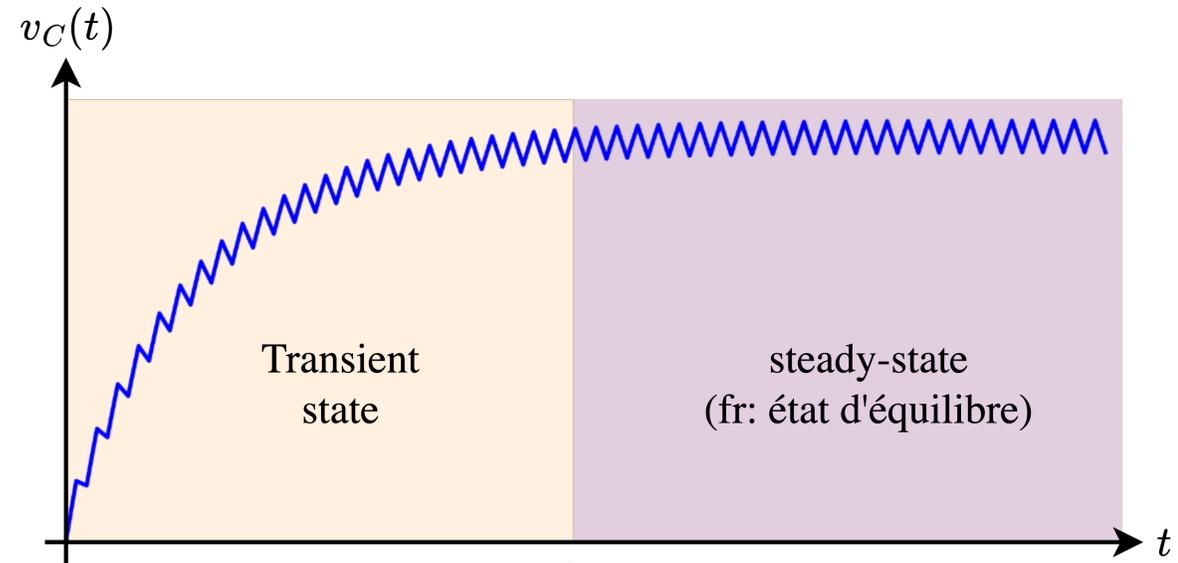
For well-chosen values of  $C$ ,  $R$ , and frequency, the RC circuit reaches a steady state in which the voltage can be decomposed into a DC component  $V_C$  and a ripple component  $v_C^{ripple}(t)$  :
