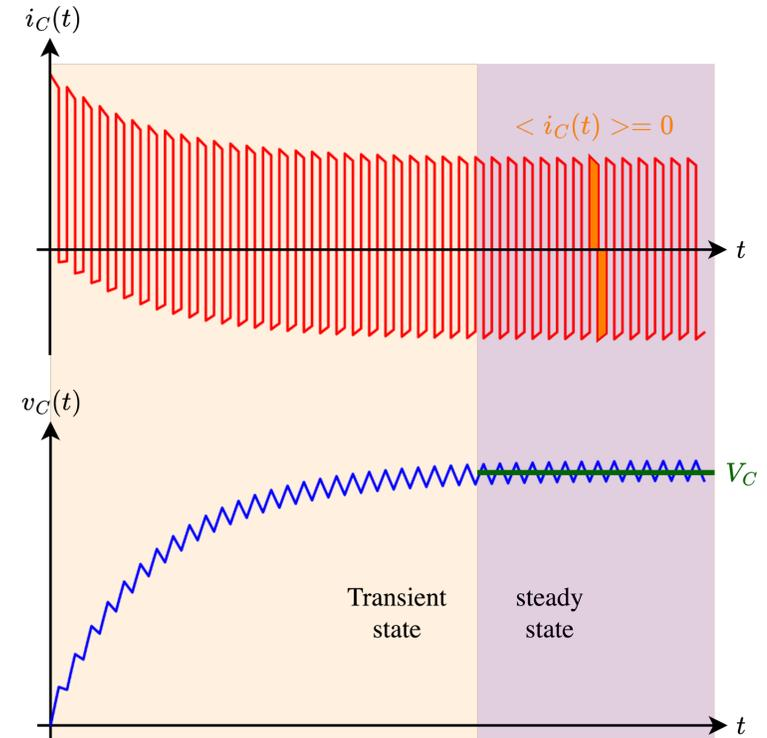
Small ripple approximation (SRA) for **capacitor voltage**
