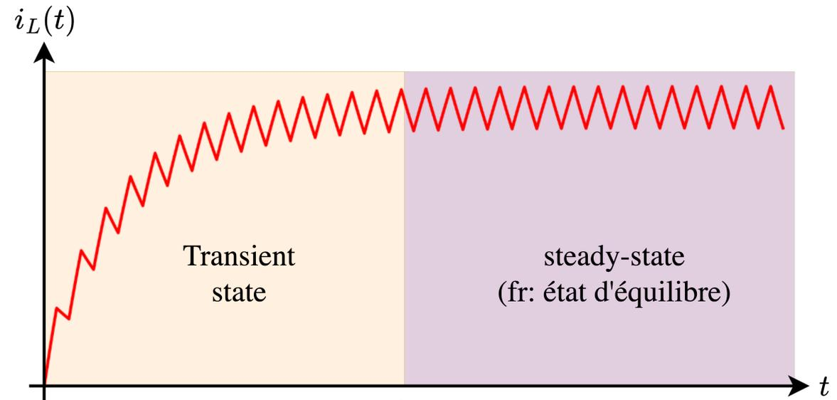
For well-chosen values of  $L$ ,  $R$ , and frequency, the RL circuit reaches a steady state in which the current can be decomposed into a DC component  $I_L$  and a ripple component  $i_L^{ripple}(t)$  :
