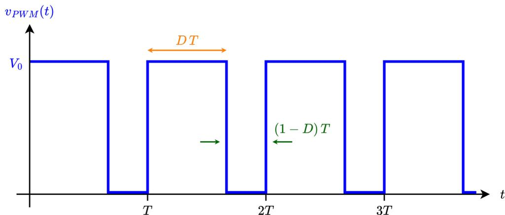
$$v_{PWM}(t) = \begin{cases} V_0 & \forall t \in [nT; nT + DT] \\ 0 & \forall t \in [nT + DT; (n+1)T] \end{cases}, n \in \mathbb{N}$$
