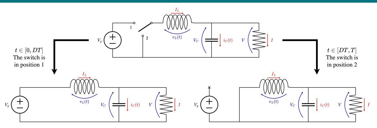
Make sure to use the same conventions in both subcircuits. The current direction MUST remain the same. The voltage direction MUST remain the same.
