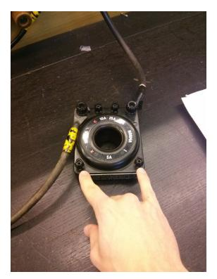
Three-phase power will be measured using the 2 wattmeters method. Use the current transformer as explained before to reduce the current range. Plug the ammeter connections in the current transformer and the voltage connections at the right place in the table. Do not forget to multiply your readings by the transformer ratio!
