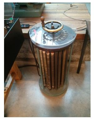
On the right side of the table. As shown on the resistors top and on the bottom picture one can see that the resistor can be adjusted from a short-circuit to an open circuit when rotating the wheel.
