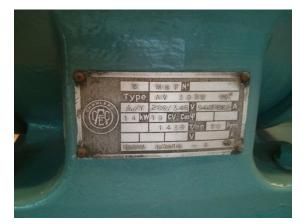
Proof that the considered motor is an asynchronous motor. What is the motor's synchronous speed ? What is the slip value at the rated speed? What about the torque? Why is the motor input connected in a "Y" configuration when starting?
