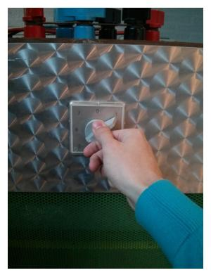
Hint: Put the autotransformer to 100% and choose the right configuration (Y or  $\Delta$ ) for primary and secondary to maximize the output voltage. You do not have to perform the short circuit test, just interpolate graphically your results.
