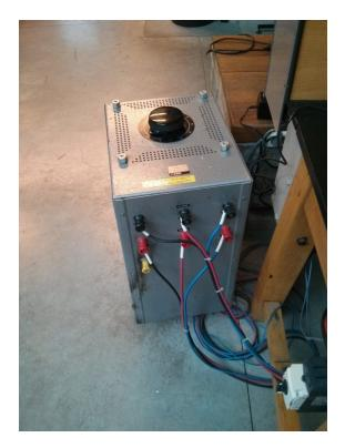
This allows to deliver an output voltage whose value depends on the angular position of the black indicator on top. This output voltage is the input voltage of the primary winding of the studied transformer. Load connected to the transformer's secondary winding:
