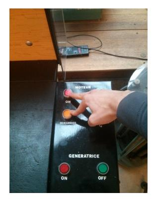
Anf finally, after the motor is started, start the generator by pressing the "génératrice ON" button and connect the excitation circuit by pressing the button on the picture.
