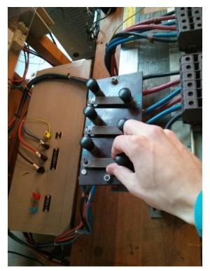
Do not forget to start the short-circuit test with 0% at the autotransformer and do not forget to take into account the Y and delta voltage ratio to guarantee to keep  $I_{out}$  lower than the rating.
