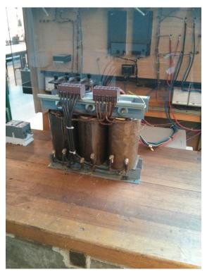
The voltage is supplied through an autotransformer:
