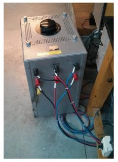
This allows to deliver an output voltage whose value depends on the angular position of the black indicator on top. This output voltage is the input voltage of the primary winding of the studied transformer. The load is connected to the DC generator's output. It allows to electrically change the asynchronous motor's load torque:
