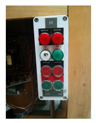
Then, start the DC motor. It will start in 3 audible steps by progressively increasing the motor's input voltage. Please set the excitation current  $I_e$  to the maximum before starting to limit the in-rush current.
