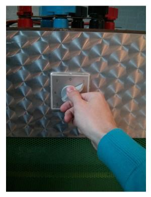
On the right side of the table. When on "0" the secondary winding is an open circuit. When on "1" it is  $27 \Omega$ , "2" is  $27/2 \Omega$ , "3" is  $27/3 \Omega$ ,... The secondary winding can not be shorted using this technique. A manual short-circuit on the back side of the table is required. All the power measurement are performed using a power quality analyzer (Fluke 434 or equivalent):
