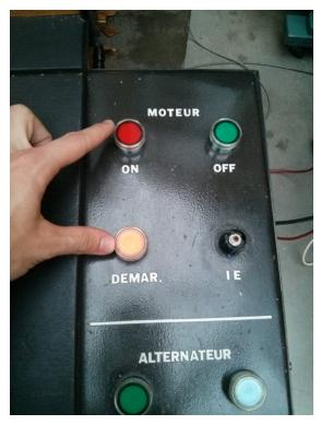
Finally, press on "charge", this will connect the load to the synchronous generator's output, then press "on". **DO NOT** press "reseau" as the generator's output is not close to the networks voltage and frequency yet.
