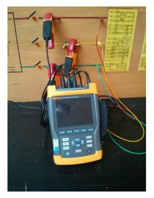
Do not forget to choose the phase coupling mode: "Y" or "Delta" configuration. Also, pay attention to the power flow direction when installing the clamps.
