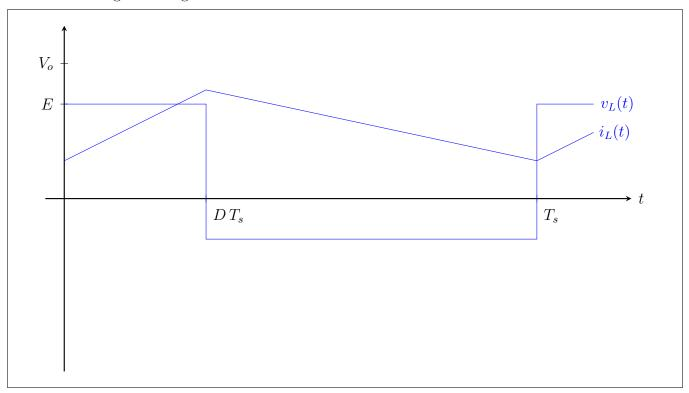
The converter is connected to a 24 V battery and is controlled at a switching frequency f = 2 kHz. With a duty cycle D of 30 %, what should be the value L of the inductor to obtain a current ripple of 100 mA?
