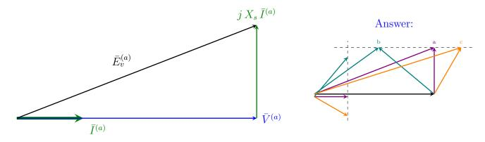
If the output active power and the RMS output voltage are kept constant, complete the above phasor diagram for two other working points:
