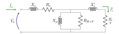
The above schematic presents the one-phase equivalent electric circuit of a three-phase asynchronous motor in star configuration. This motor has three pairs of poles, and is powered at a frequency of 60 Hz.
