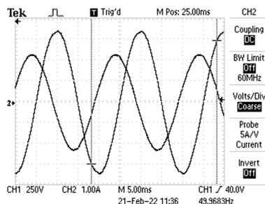
Phase voltage and corresponding phase current at the input of an asynchronous machine powered by a three-phase power supply.
