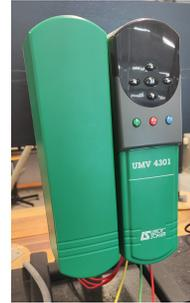
An electrical box connects the speed controller to the asynchronous motor. In particular, the yellow, green and red banana connectors hold the three-phase voltages generated by the speed controller and supplying the asynchronous motor. **Do not unplug them if the table is on.**
