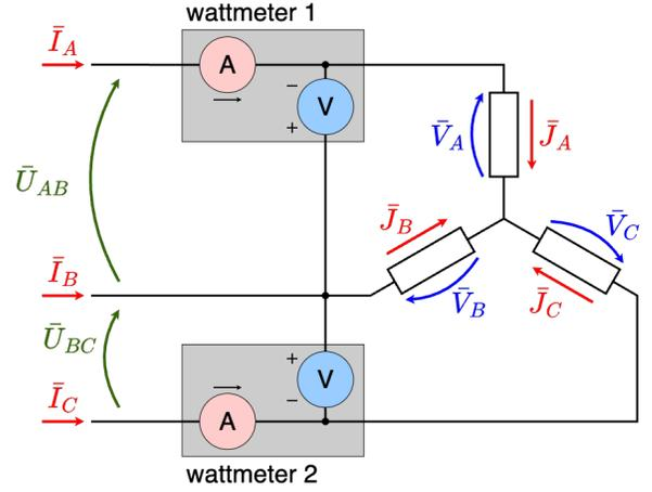
In this configuration, the voltages and currents can be represented on a phasor diagram. Taking  $\bar{U}_{BC}$  as the reference,  $\bar{U}_{AB}$ ,  $\bar{U}_{BC}$ ,  $\bar{J}_A$  and  $\bar{J}_C$  can be expressed as:
