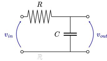
This low-pass filter reduces high-frequency components but also introduces a phase shift (see figure below).
