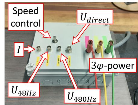
Four coaxial connectors allow to measure the following signals:
