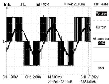
Voltage and current at the output of the speed controller.
