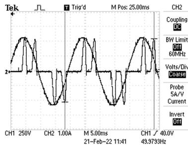
Voltage and current at the input of the speed controller.
