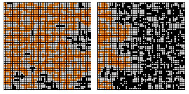
Figure 2: Examples of conducting grid (left) and non-conducting one (right). Grey cells are made of non-conducting (matrix) material, black cells are made of non-connected conducting material and orange cells are mode of connected conducting material.
