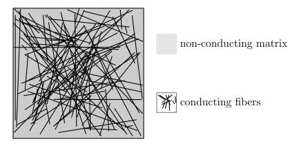
Figure 1: Example of a composite material made by non-conducting matrix with conducting fiber. This is this structure that will be study in this project.
