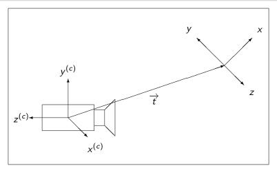
$$\begin{pmatrix} x^{(c)} \\ y^{(c)} \\ z^{(c)} \end{pmatrix} = R_{3\times3} \begin{pmatrix} x \\ y \\ z \end{pmatrix} + \begin{pmatrix} t_x \\ t_y \\ t_z \end{pmatrix}$$
